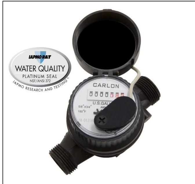
The SJM® single jet series meter is tested and certified to NSF/ANSI 372 for lead free compliance. This robust meter is suitable for reverse osmosis, de-ionized, hot (160°F), or cold water. The SJM® meter can handle up to 232 psi and the sealed register has the ability to rotate 360°. The meter has an integral strainer and is offered in gallons or liters.
