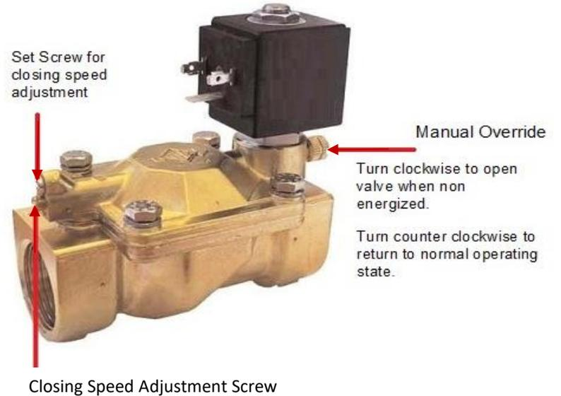
Thread into the valve in a clockwise rotation until desired closing speed is found
