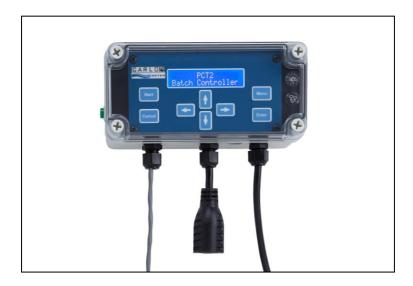
Carlon's PBC® Programmable Batch Controller provides a means for automatically measuring the amount of water desired for a batch. The PBC® eliminates the need for manual measurement and assures the proper water volume each time. The PBC® has a start button mounted on the outside box; this way once the batch size is entered the box can be closed and there is no need to reopen the box unless the batch size is being changed.
