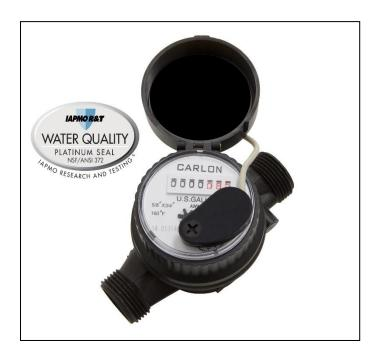
The SJM<sub>®</sub> single jet series meter is tested and certified to NSF/ANSI 372 for lead free compliance. This robust meter is suitable for reverse osmosis, deionized, hot (160°F), or cold water. The SJM<sub>®</sub> meter can handle up to 232 psi and the sealed register has the ability to rotate 360°. The meter has an integral strainer and is offered in gallons or liters.
