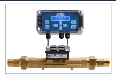
The Ultrasonic Meter series (USM<sub>®</sub>) has a wide temperature range with a high degree of accuracy. The remotely mounted register displays total volume and can display a momentary "Real Time" flow. The USM<sub>®</sub> Series provides a selectable dry contact pulse output. This unit is designed for heating and cooling systems.
