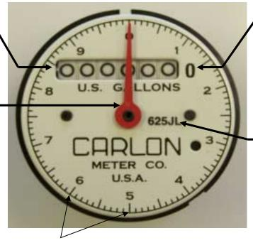
1 gallon increments for 5/8", 3/4", and 1" meters or 10 gallon increments for 1 1/2" and 2" meters
